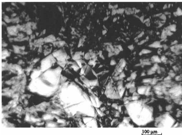
FIGURE 2 Optical micrograph of the carbon foil (based on graphite compound with high crystallinity –type 2).
